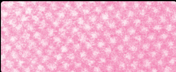
Roller / Nip Defects, Parallelism / Crown Correction Problems
