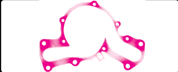
Uneven / Insufficient Loading
