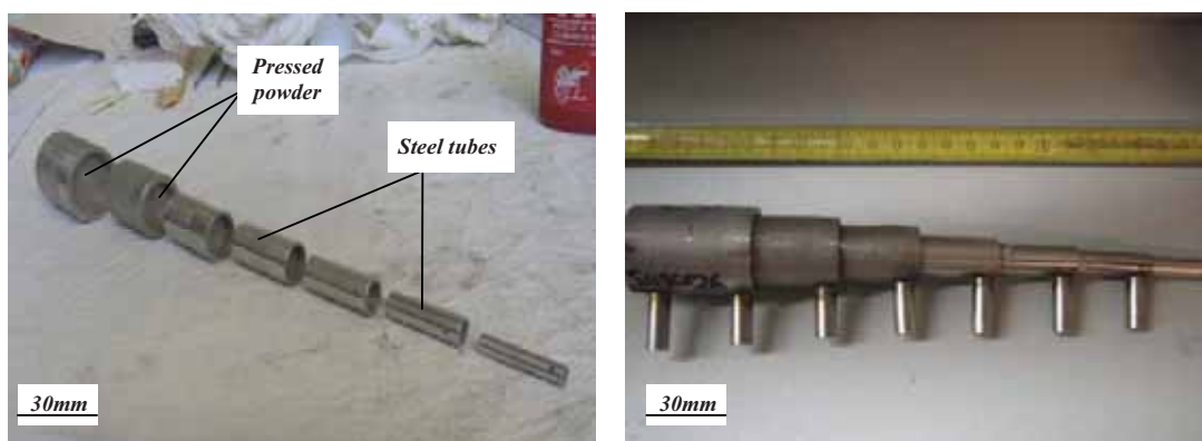
Figure 4.4: Detail of a seven tubes configuration for combustion front tests: cold uniaxial pressing of initial powder mixtures is achieved (left), tubes are coupled in order to form the stack of cylinders considered in configuration 1 (right).
