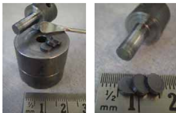
Figure 5.5: Photographs of the steel die and \text{Al} / \text{MoO}_3 pellets after cold uniaxial pressing. In order to achieve highly dense greens, the upper punch of the steel die was hardened to avoid deformations while pressing.
