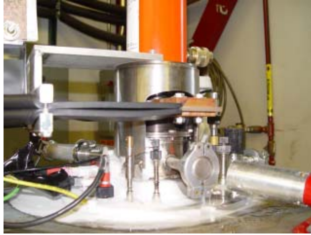
Figure 3. Strain device ready for test in the cryostat.
