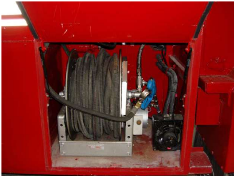
Figure 3.3.11: The UHP P-19's UHP hand line reel.
