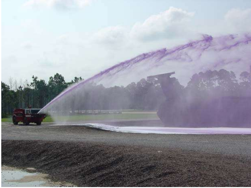
Figure 4.5.4: 300 gpm combined agent Williams Hydro-Chem™ bumper turret nozzle being used to conduct a combined agent throw test.
