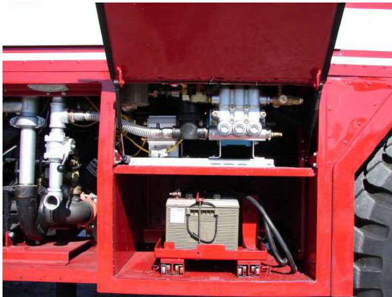
Figure 3.4.1: UHP P-19 Foam proportioning system (top) and battery (bottom).
