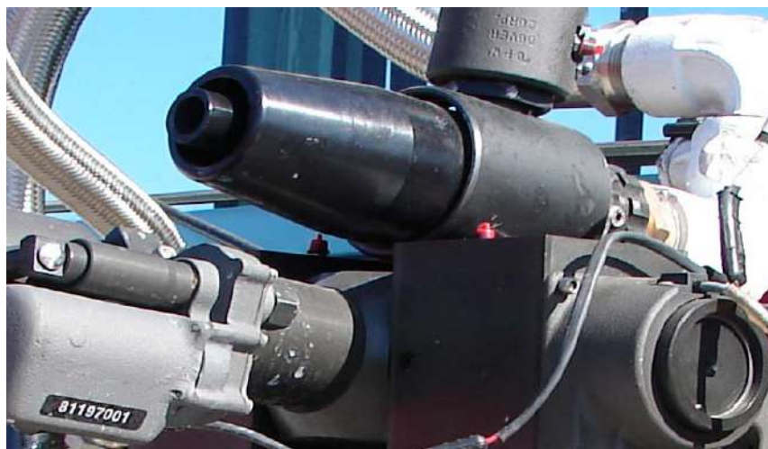
Figure 3.5.1: A 300 gpm combined agent Williams Hydro-Chem™ nozzle mounted alongside the Elkhart Brass UHP bumper turret.
