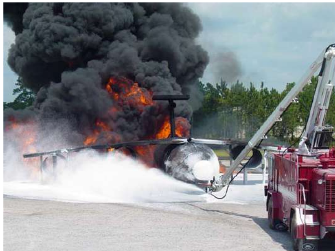
Figure 2.4.2: The 200 gpm UHP T-1500 Extinguishing a 7000 ft 2 pool fire.
