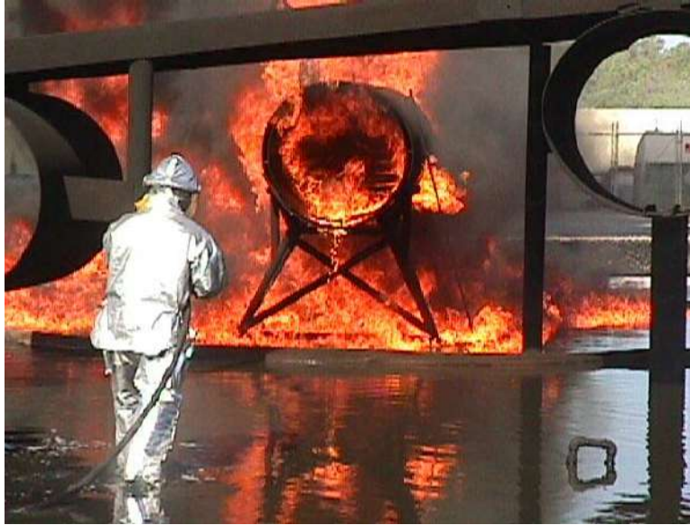
Figure 2.1.1: 3-D foam application to a 3-D flowing fuel fire.
