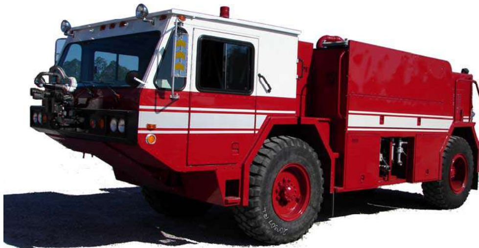
Figure 3.2.1: The retrofitted UHP P-19 ready for duty.
