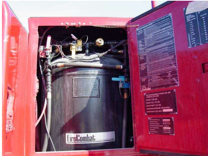
Figure 3.6.1: The 500 lb dry chemical storage tank located behind the passenger's side cab.
