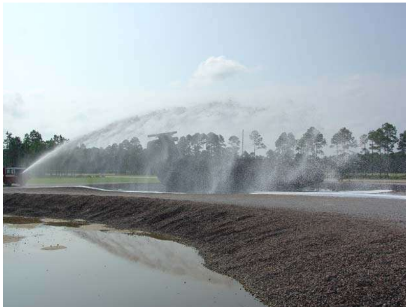
Figure 4.5.3: 300 gpm combined agent Williams Hydro-Chem™ bumper turret nozzle being used for a compressed air foam throw test.
