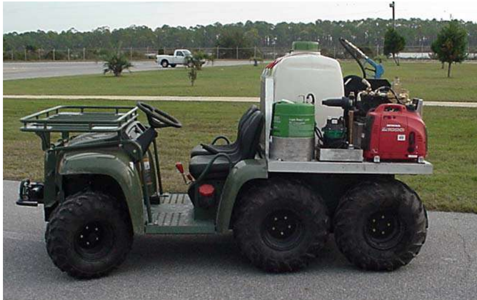
Figure 2.2.1: Side view of the 14 gpm FRE vehicle with optional equipment.
