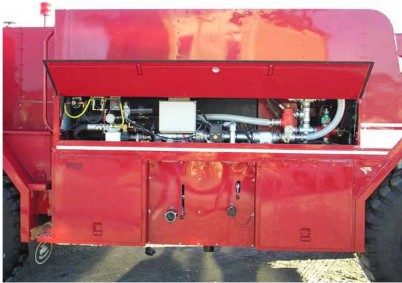
Figure 3.3.10: The UHP P-19's driver's side plumbing.
