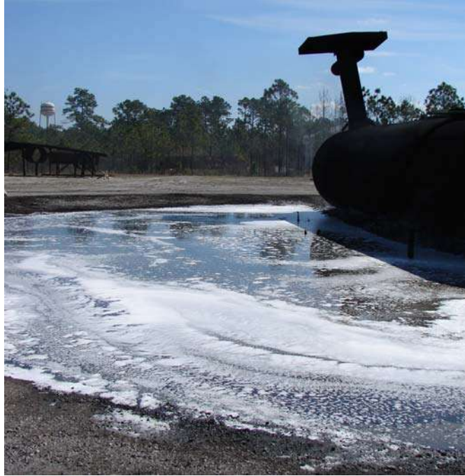
Figure 4.6.6: The foam blanket produced in preparation for burn back testing after extinguishment of a 3500 ft 2 fire with the UHP P-19.
