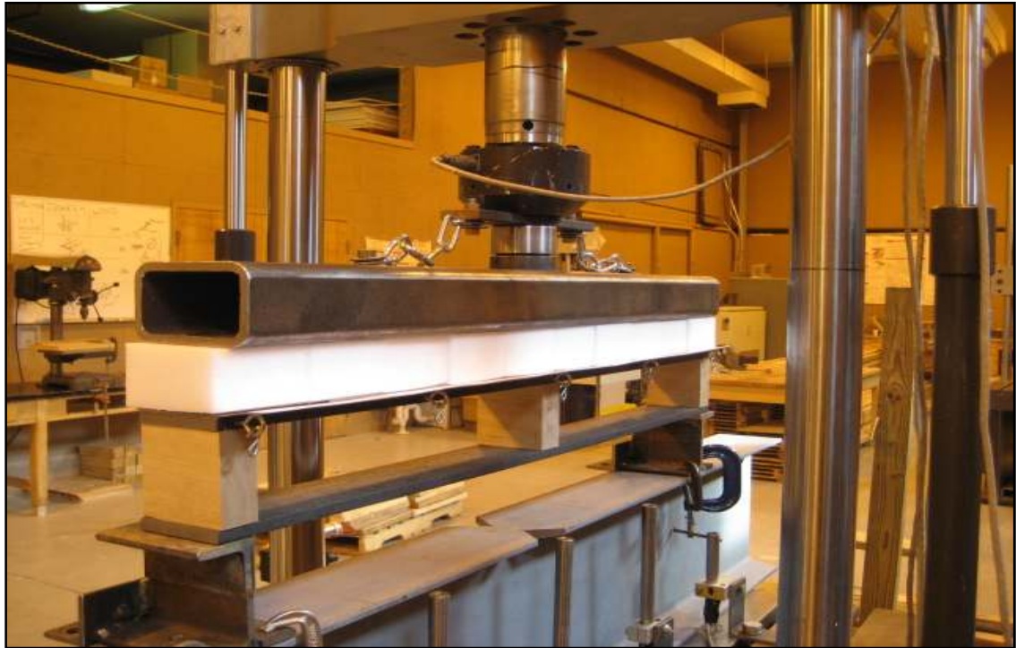
Figure 3.2 Testing setup for a simulation of pallet storage rack.
