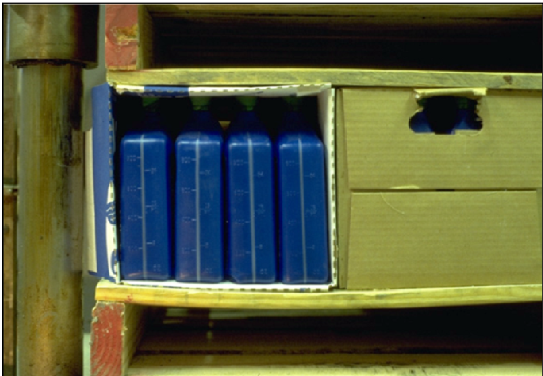
Figure 1.2 Non-uniformly distributed loads on packaging and pallet.
