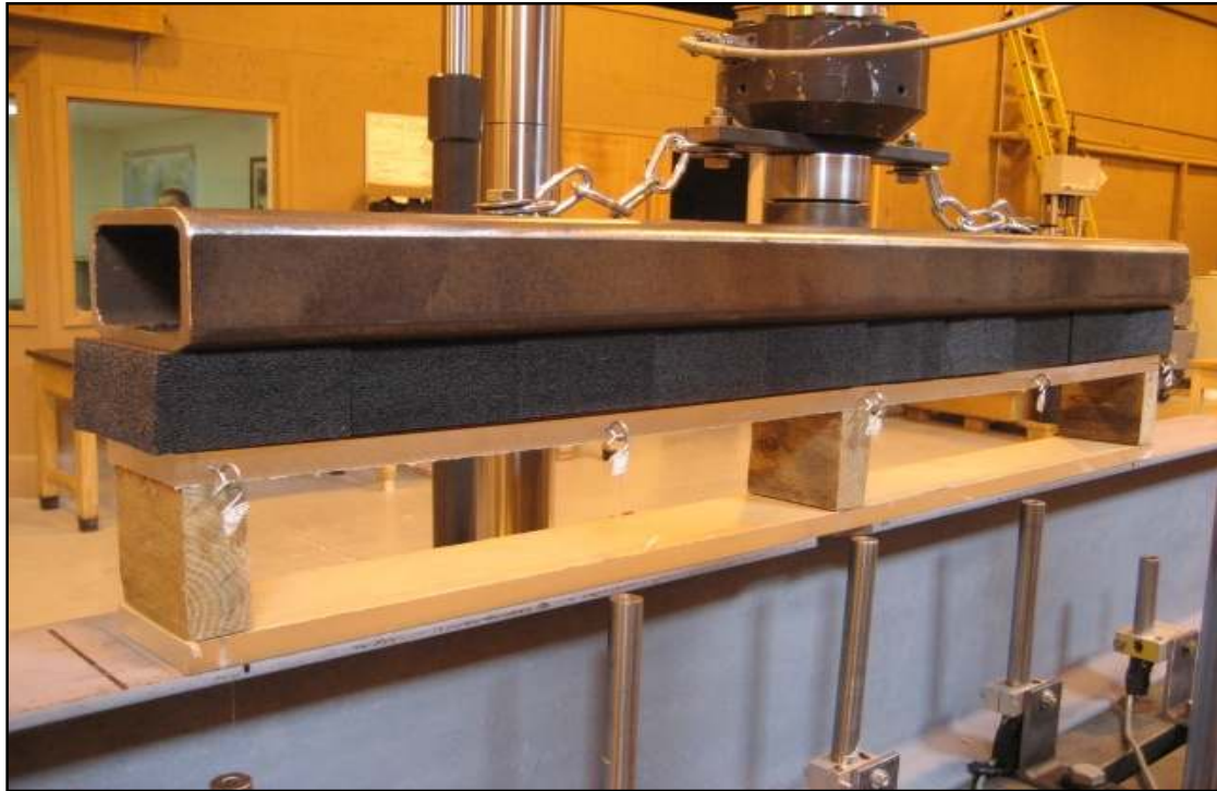
Figure 3.4 Testing setup for a simulation of block stack storage system.
