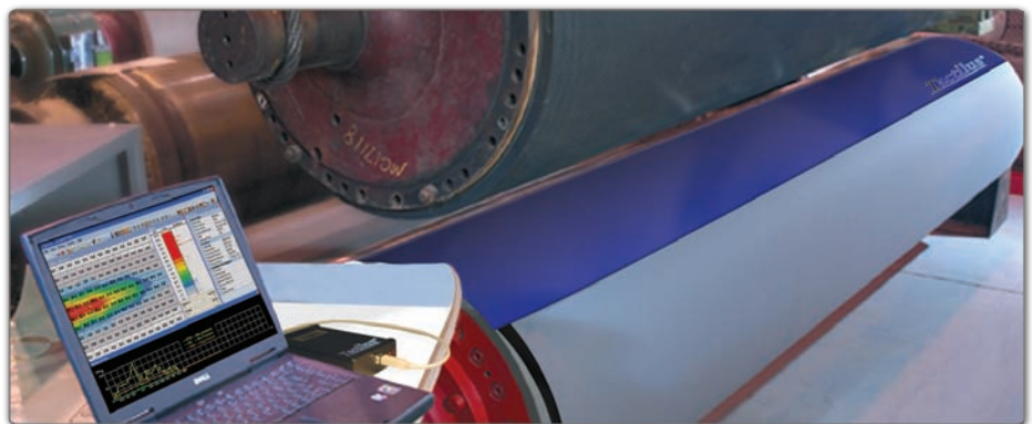
Actual sensor positioned on a nip ● Tactilus® software displayed on laptop
