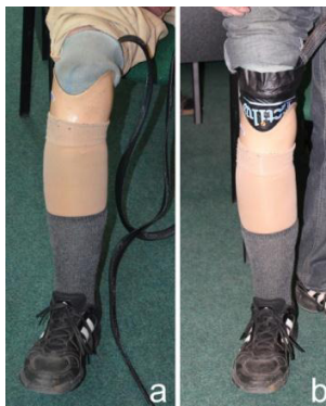
Fig. 2 Pressure sensor placement methods- a)stump/liner, b) liner/socket
