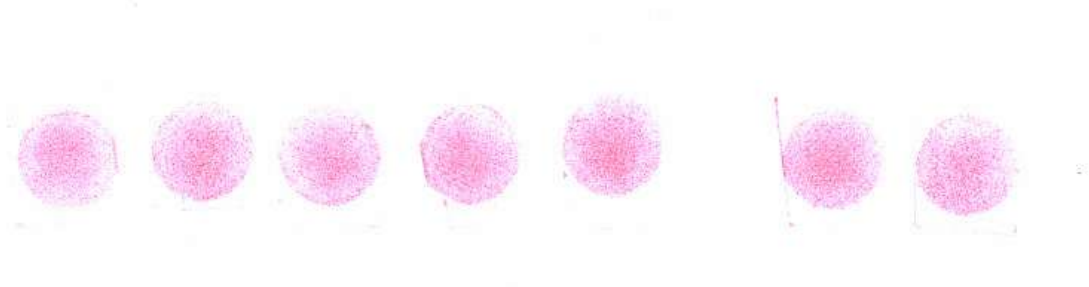
Figure A.5: Pressure film impressions made during a repeatability test on the Instron material testing machine at a target pressure of 0.477 MPa (70 psi.).
