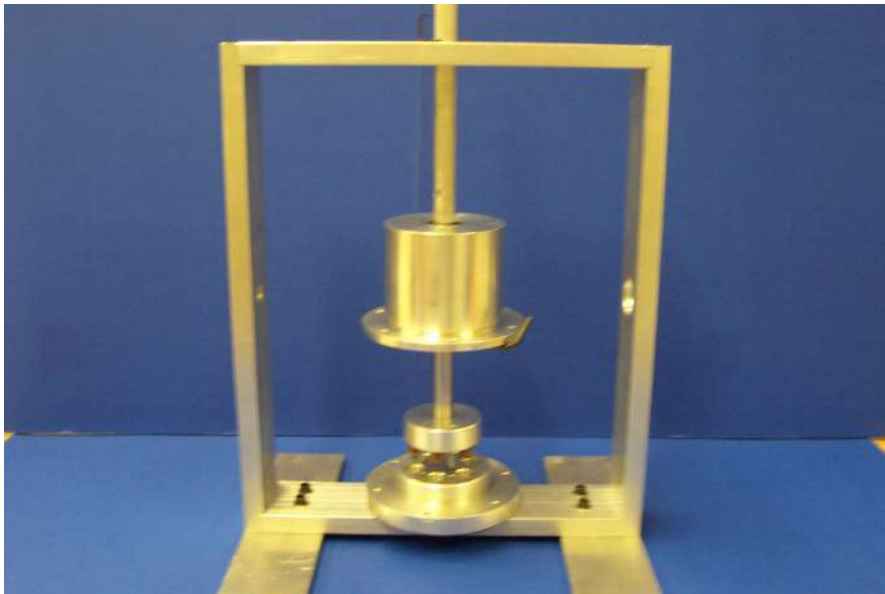
Figure B.1: A picture of the setup frame assembled with the dish, plunger, and cap showing arrangement of fixture during sample loading and unloading.
