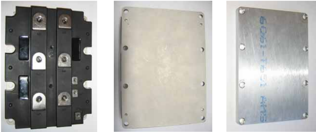
Figure 4-1: Power Electronics Module: Top (left), Bottom (center), and Test Heat Sink (right)
