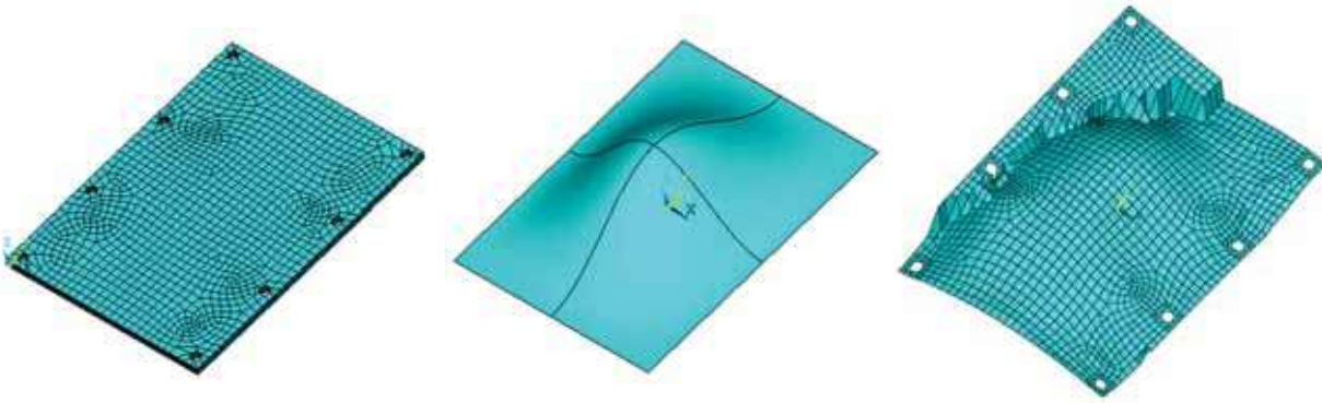
Figure 4-3: Base Plate Surface Models: Flat (left), Sinusoidal (center), and Imported (right)
