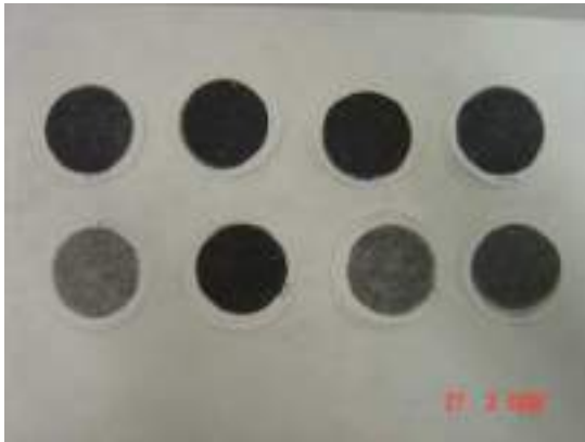
Figure 3.19. Lint After Being Filtered for Weight Analysis
