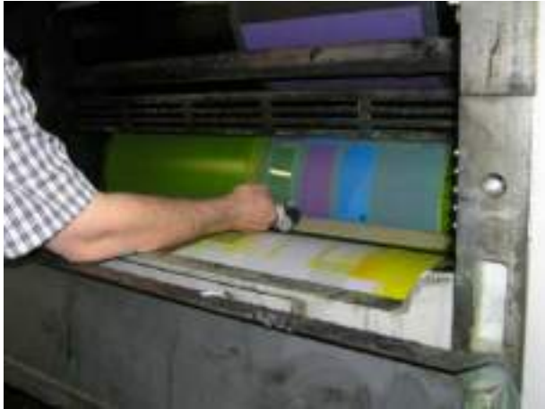
Figure 3. 15. Application of Tape to the Blanket
