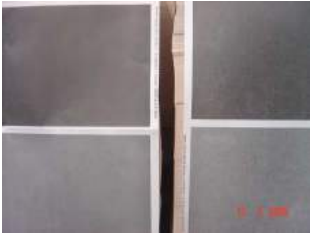
Figure 2. 4. Image Degradation from the beginning of the run (LHS) to the 7000th copy (RHS) caused by linting.
