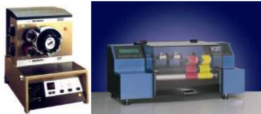
Figure 3. 2. IGT printability tester AIC2-5 printing unit [82] and IGT printability tester AIC2-5 inking unit. [73].
