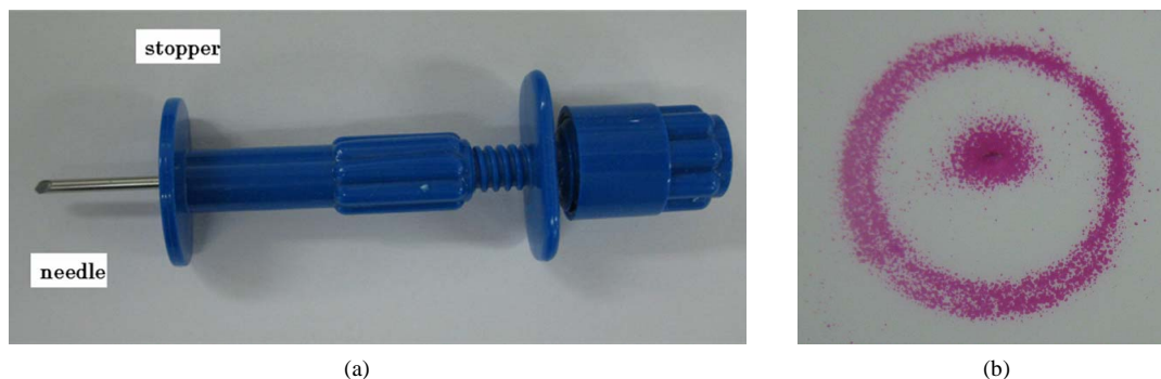
Figure 1. (a) Bone marrow aspiration needle: In this paper, we used two kinds of needles for bone marrow puncture purchased from CareFusion Japan (DIN1518X, 15 G; Tokyo, Japan) and TSK Laboratory (SIL-151, 15 G; Tochigi, Japan). Hematologists (Table 1) performed the bone marrow puncture on wood using a needle purchased from CareFusion Japan, as shown in (a); (b) Pressure sensitive film showing the contact pressure from bone marrow puncture: The Fuji Prescale medium grade pressure-sensitive film with a pressure range of 10 - 50 MPa was used for measuring contact pressure. Hematologist #2 (Table 1) performed the bone marrow puncture on wood using a needle purchased from CareFusion Japan (a). Contact pressure changed the color on the prescale film from the white to pink, or red color dependent on the grade of pressure. Pressure changes were noted at the needle area (center position) and at the stopper area (around the needle area).
