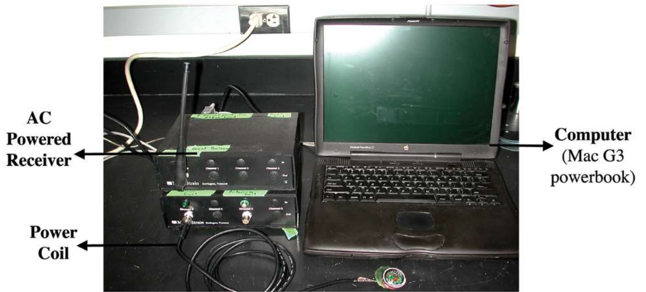
Figure 2. Computer Based Measurement System showing a Macintosh G3 powerbook (right) connected to the AC powered receiver via a serial cable and the power supply for the coil that inductively powers the transmitter.
