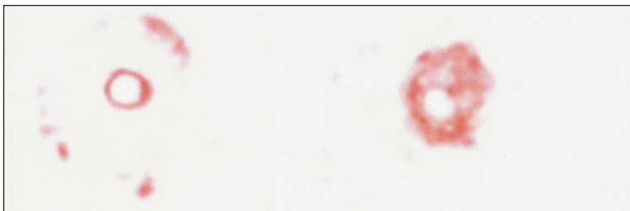
Fig. 2 Scanned image of Fuji PresSurex film after compression. Coloured regions indicate areas of compression generated across the fracture surface. The image on the left is the scanned image of the Fuji PresSurex film after compression of the right humeri using the Orthofix pin method. The image on the right is a scanned image of the Fuji PresSurex film after compression of the left humeri using the lag screw method.
