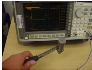
Figure 3: Dynamic Signal Analyzer (above) and Calibrated Hammer (below)
