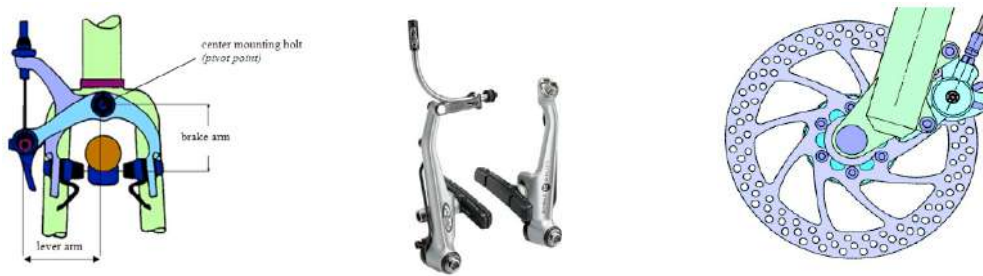
Fig. 1- left to right: side-pull caliper brake (rim brake) for road bikes with one centred mounting bolt; V-brake (rim brake) for city-, trekking- and mountain bikes; a disc brake (hub brake) for mountain bikes mounted by IS2000 standard [2]
