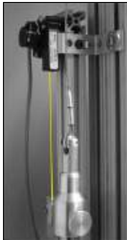
Figure B-3: A linear position transducer was mounted on the tracking 80/20 to measure cable excursion.
