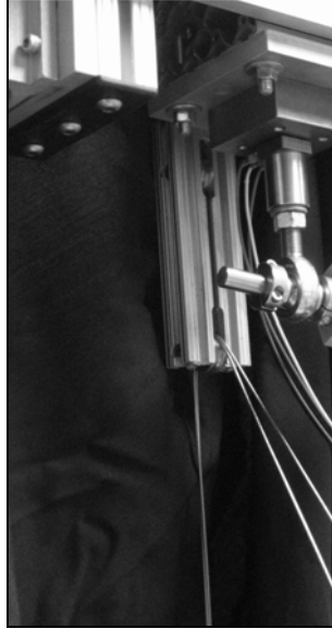
Figure B-7: A pulley housed within a section of 80-20 15 series was rigidly attached to the pelvic block. The pulley represented the ischial tuberosity and the proximal attachment point of the hamstring muscle group. A static load was hung from the wire rope to simulate muscle force. This arrangement was utilized for the mechanical knee assembly.
