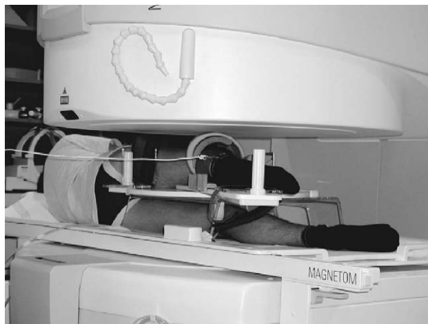
Fig. 1. Photograph showing a patient lying on his side on the MR open table. The positioning device allows for reproducible alignment of the knee flexion angle, and avoids motion artifacts during image acquisition. An external load of 3 kg, leading to a torque of about 10 Nm about the knee joint, is applied to the distal shank.
