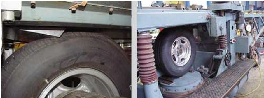
Figure 4.1: Flat plank tyre tester [3]
