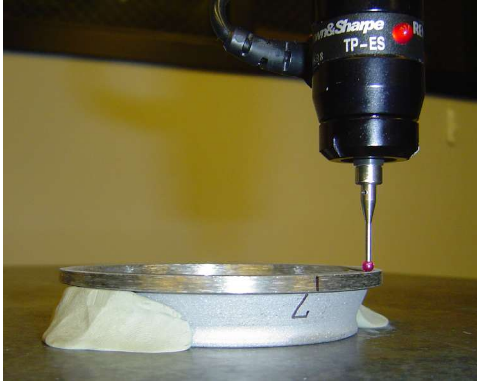
Figure 4.1: Experimental setup for measurement of initial PTV surface profile variation
