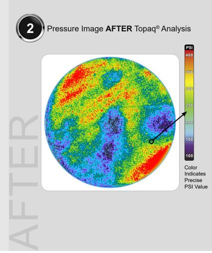
The image to the left depicts a Fujifilm Prescale<sup>®</sup> impression, while the image to the right is a color mapped version produced with the Topag<sup>®</sup> Tactile Force Analysis System.
