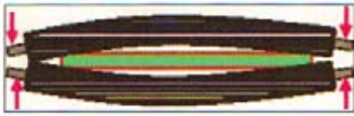
FIGURE 2. Illustration of roll bending (exaggerated).
