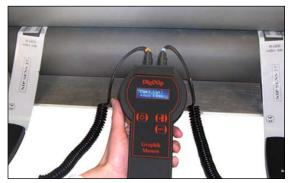
between rollers. Measurements allow real-time roller adjustments for parallelism to be made quickly and easily, extending roller life and improving product quality.
