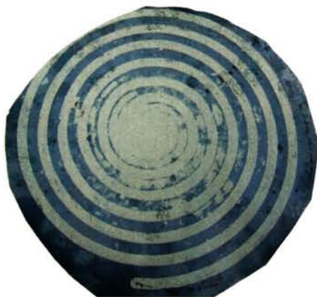
Mold-Align reveals flash in the center of the spiral mold.
