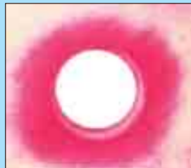
Pressure distribution across a bolted joint
