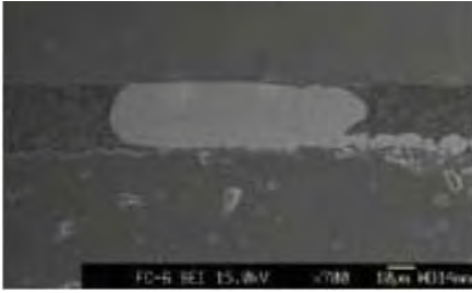
Figure 5. Cross section of a coined gold stud bump connection
