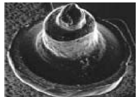
Figure 4. Gold stud bump showing wire stub at top
