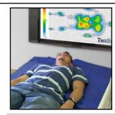
When a person sits on a seat or mattress covered with the Bodyfitter pad, its more than 1,000 sensing points measure pressure in real time and display it as 2D or 3D color-coded pressure maps.
