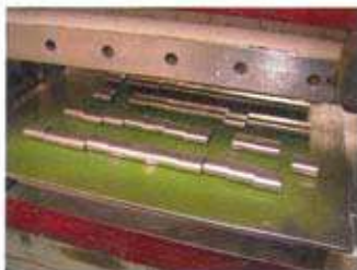
Figure 1: SB Electronics' capacitors after being pressed
