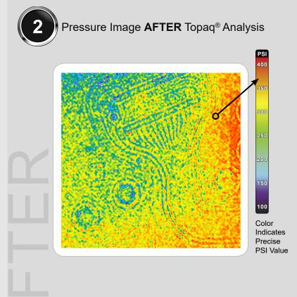
The image to the left depicts a Fujifilm Prescale® impression, while the image to the right is a color mapped version produced with the Topag® Tactile Force Analysis System.
