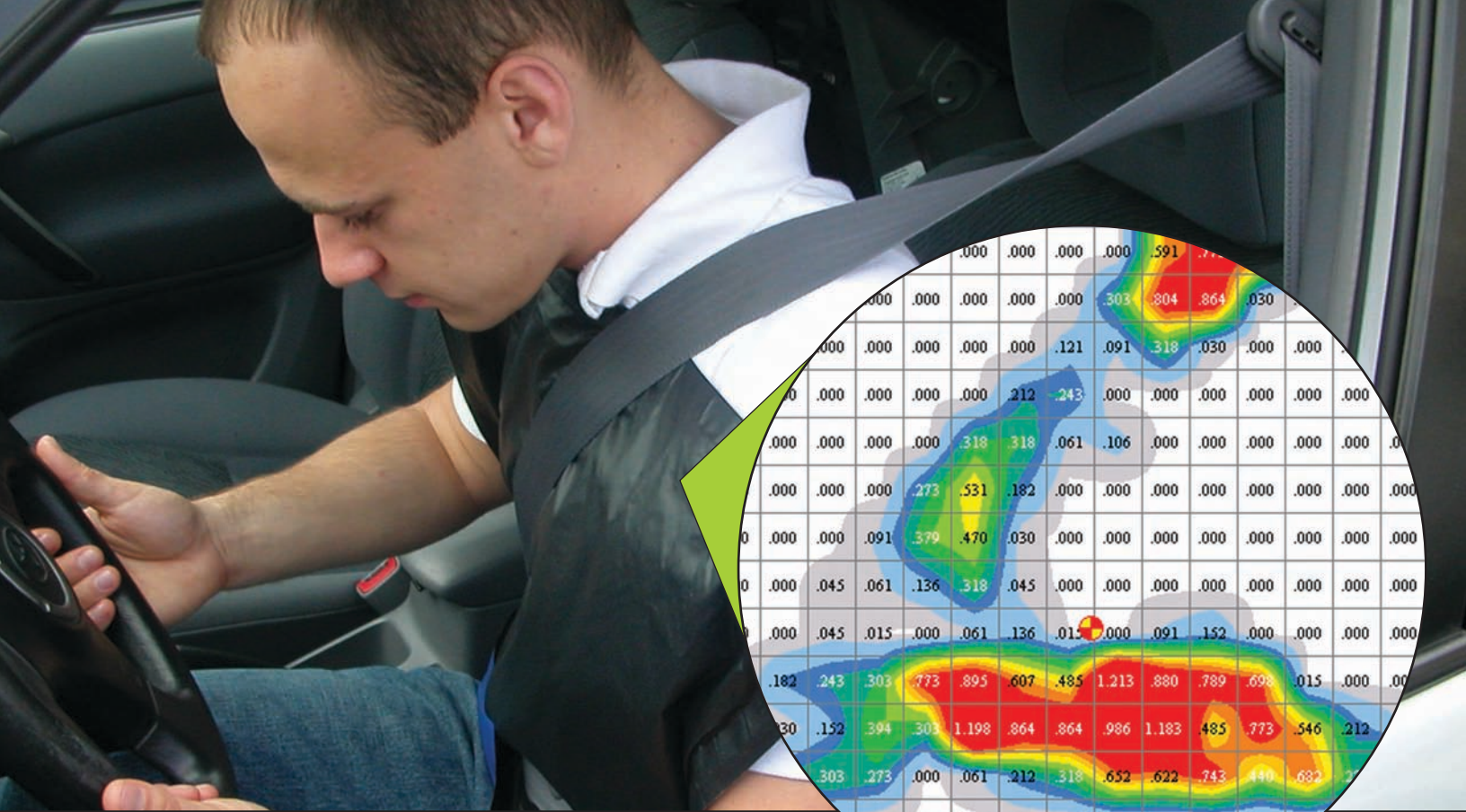
2-D view of pressure distribution during heavy braking.
