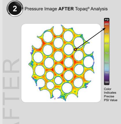
The image to the left depicts a Fujifilm Prescale<sup>®</sup> impression, while the image to the right is a color mapped version produced with the Topaq<sup>®</sup> Tactile Force Analysis System.
