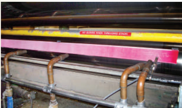
Pressurex reveals variations in nip contact pressure which can be easily quantified
