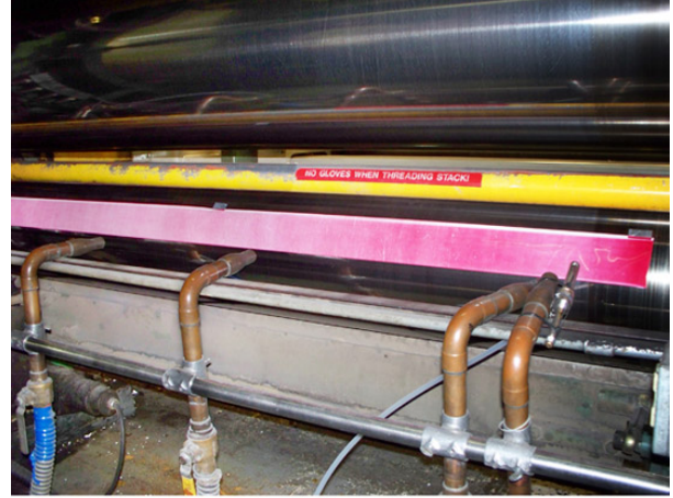
Pressurex® reveals variations in nip contact pressure which can be easily quantified.
