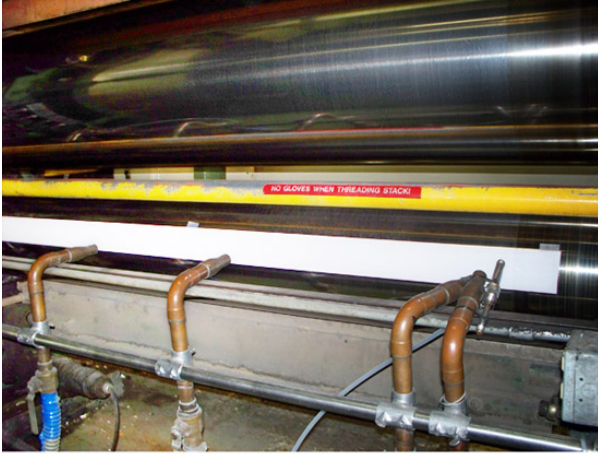
Pressurex® is placed on the roller at Mohawk Fine Papers before closing the nip.
