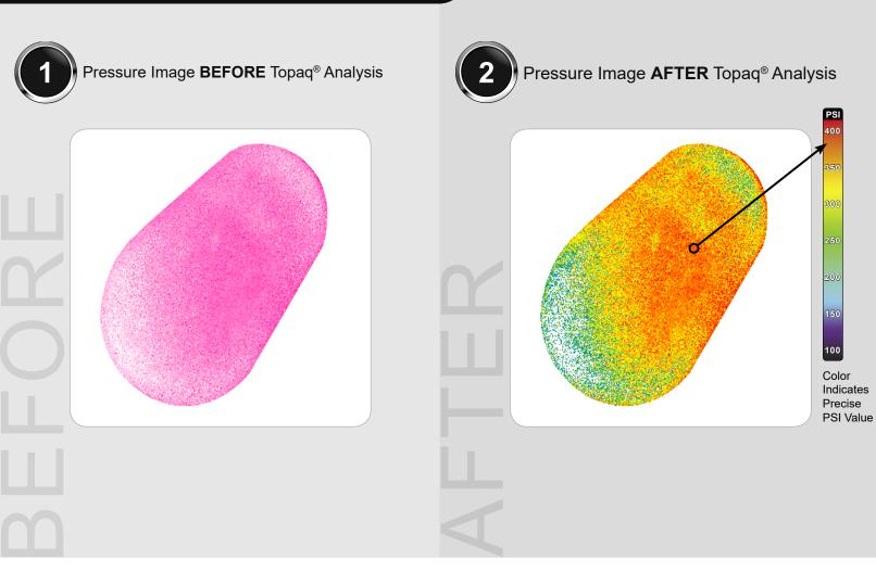
The image to the left depicts a Fujifilm Prescale<sup>®</sup> impression, while the image to the right is a color mapped version produced with the Topaq<sup>®</sup> Tactile Force Analysis System.
