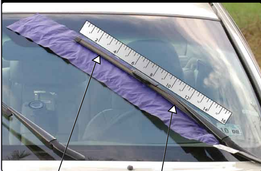
Sensor element positioned under a windshield wiper
