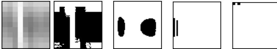
Figure 4: (a) The original tactile image, (b) threshold, (c) erosion and concave location filter, (d) horizontal CCD, (e) vertical CCD
