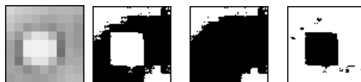
Figure 3: (a) The original hole, (b) threshold, (c) contour, (d) the hole
