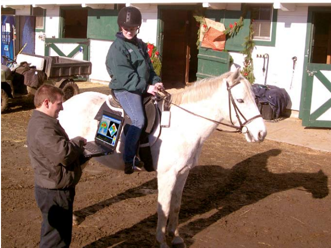
Equestrics® Sensor instantly reveals rider's pressure on saddle.
