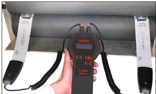
DigiNip® sensor elements placed between two contacting rollers
