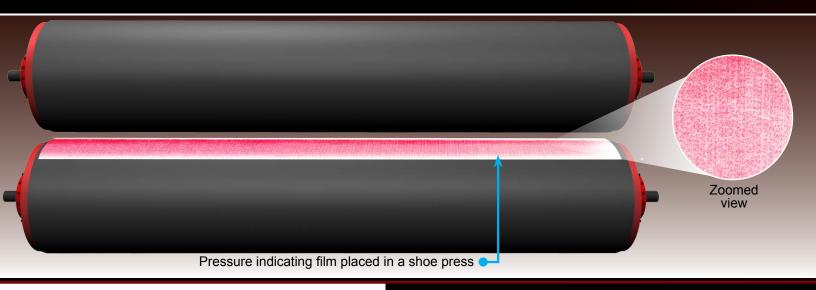
The Shoe Press Profiler® easily allows any technician to quickly and easily capture an extremely high resolution pressure reading of the shoe press. Used on conjunction with pressure indicating films, the Shoe Press Profiler® provides instantaneous and intuitive reports that reveal a wealth of statistical data about your pressure profile. Unlike other pressure systems there is no complicated calibration nor extensive expertise required for replacement of the sensor system.
