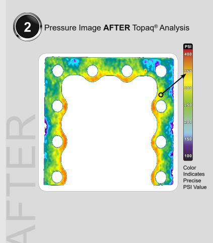
The image to the left depicts a Fujifilm Prescale® impression, while the image to the right is a color mapped version produced with the Topag® Tactile Force Analysis System.
